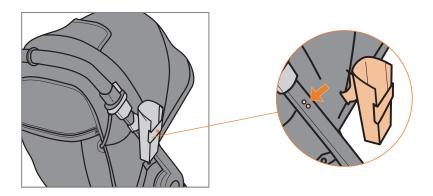
Remove the current cup holder from the frame. The new cup holder can be attached to either the left or right side. Align cup holder bumps with the corresponding holes on the handlebar tube. Pull down on the cup holder to confirm it is secured in place.
