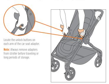
Press the button on each arm and pull the car seat adapter away from the stroller.
