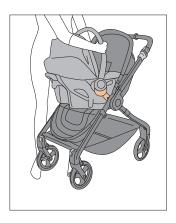
Pull each side of the car seat handlebar upward to verify the installation is secure. The car seat should be firmly attached to both sides of the car seat adapter.
