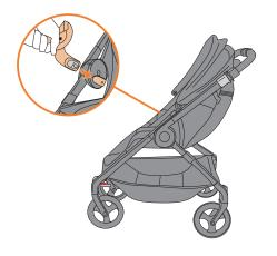
Position the handlebar of the stroller in the Forward-Facing position as shown. Align each arm of the car seat adapter with the docks on the central hubs of the stroller.
