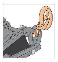
Confirm that the new wheel matches the letter on the current wheel and on the respective stroller mount (A - A and B - B). Insert new wheel into stroller opening until you hear an audible "CLICK". Pull on wheel to confirm wheel is securely installed.
