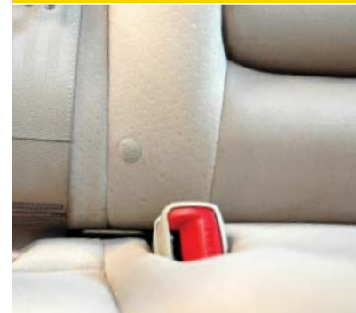
Close-up of typical Lower LATCH anchor, usually found in the vehicle seat crease.
